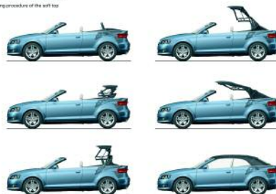
Audi A3 Cabriolet Folding operations of the soft top
